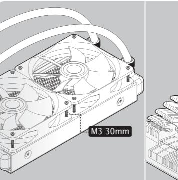
Use 30mm screw 8pcs to install Fan on radiator. Use 6mm screw 8pcs to install radiator on the top of PC case or other position. Use screw driver to fasten the 2 screws finger tight on AIO device to the Intel / AMD clip in a rotation.
