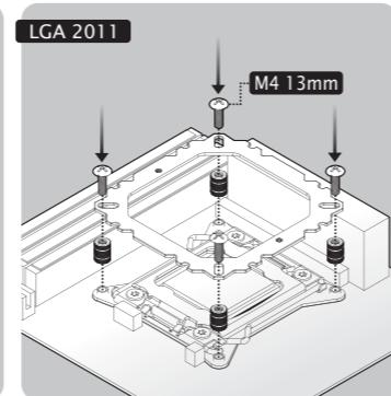
Install material M4 screw 4pcs, Metal nut 4pcs, Washer 4pcs, Back plate on the back of Motherboard. Use 4pcs M4 Screw to fasten INTEL clips.
