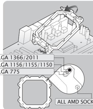
Before installation please remove original CPU Cooler or other stand from CPU. Before installation, check the hole position of M/B.
