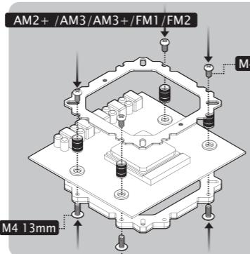
Install material M4 screw 4pcs, Metal nut 4pcs, Washer 4pcs, Back plate on the back of Motherboard. Use 4pcs M4 Screw to fasten AMD clips.
