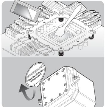
Please clean the surface of CPU before apply Thermal grease and use Plastic brush even the grease on CPU.
