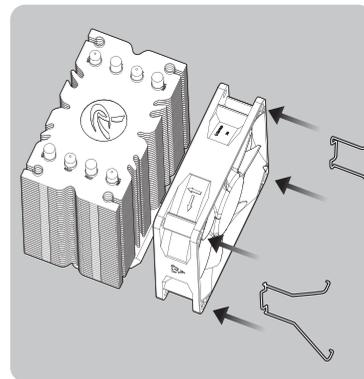
Insert fan clips onto holes of fan. Utilize fan clips to buckle fan securely onto heat-sink.
