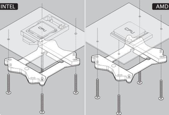
Aim the holes of back plate to the holes of MB, then let Knurled threaded screws through back plate and MB
