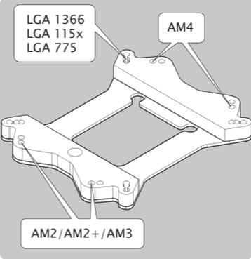
Before installation, check the hole position of M/B; Intel LGA775, LGA115x or LGA 1366; AMD AM2, AM2+, AM3 or AM4.
