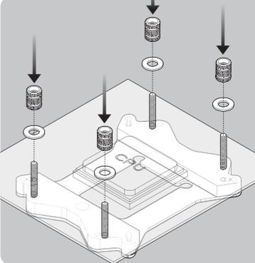
Use metal nuts to fasten back plate and MB
