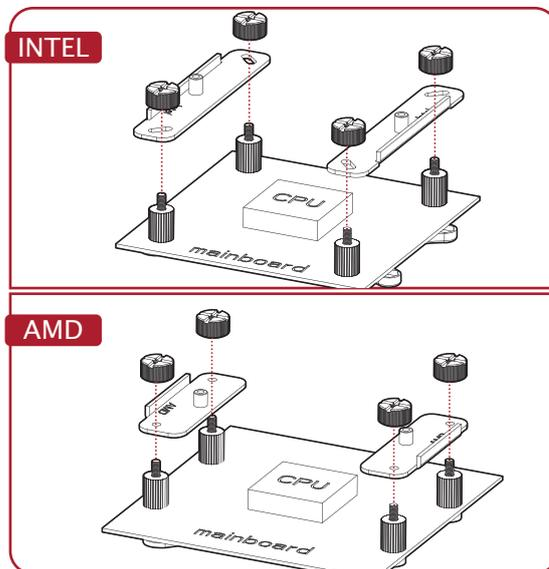
Then, aim the holes of mounting-clip to the Knurled threaded screws, then slip over the clips to the screw, and use metal nuts to fasten.
