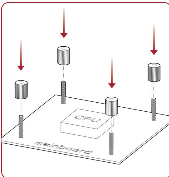
Use plastic nuts to fasten back plate and MB
