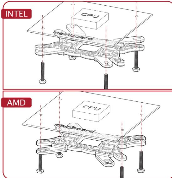
Before installation, check the hole position of M/B; Intel LGA775, LGA1155/1156/1150 or LGA 1366; AMD AM2, AM2+ or AM3.
