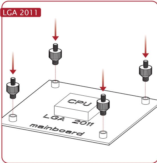
Fasten LGA 2011 screws tightly onto MB.
