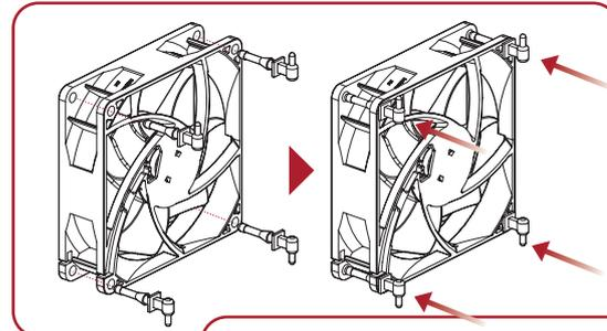
Securely fix the anti-vibration rubbers onto the fan.
