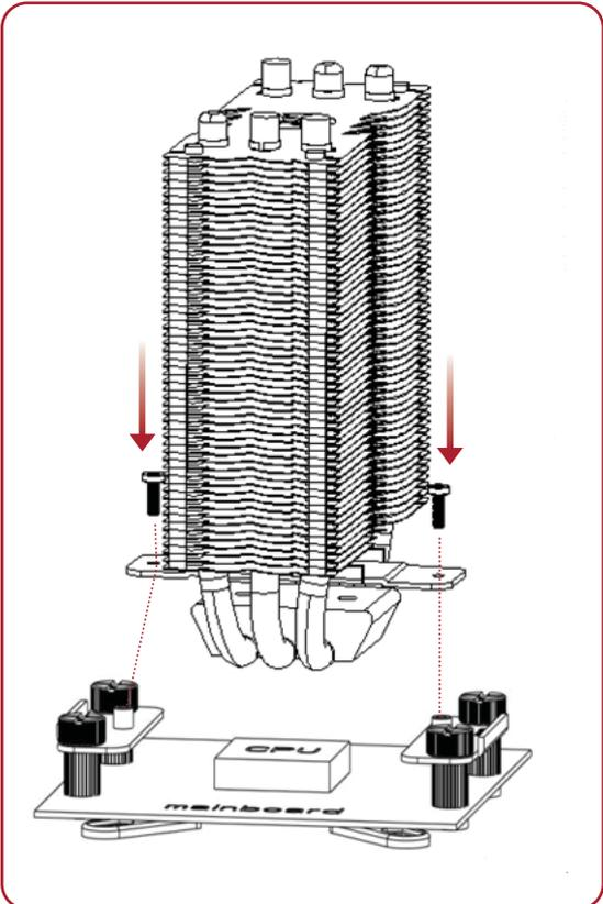
Aim the holes of crossbar to the pillar holes of mounting-clip, then use screw driver ⊕ and M3 screws to fasten cross bar and mounting-clips.
