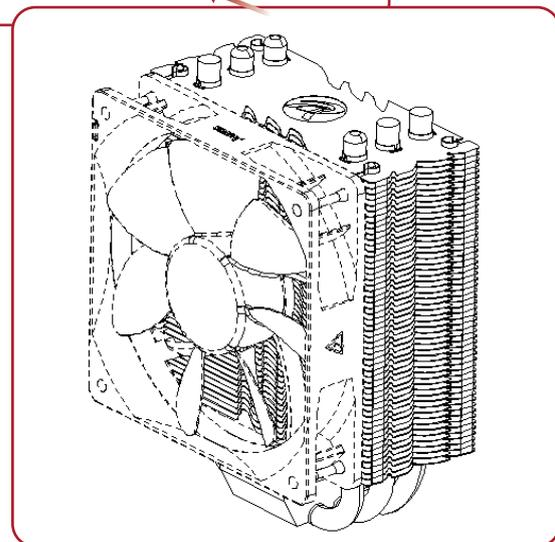
Insert anti-vibration rubbers into Heatsink (insert through form top of fins). Then, insert anti-vibration rubbers into Heat-sink (insert through from bottom of fins).
